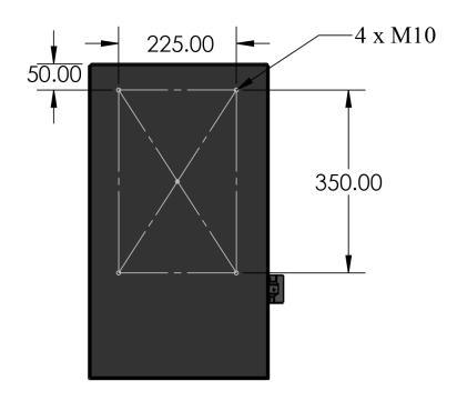
Dimensions are in millimeters
