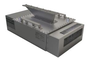
RAXON200LPB is an industrial X-ray source for producing a beam of high intensity X-rays with small focal spot and high stability which ensures uniform beam intensities and dose rate throughout its fan/cone-shaped beam. Stable voltage and electrical power applied to X-ray tube, guarantees stable dose exposure and high-quality images in digital radiography applications.
